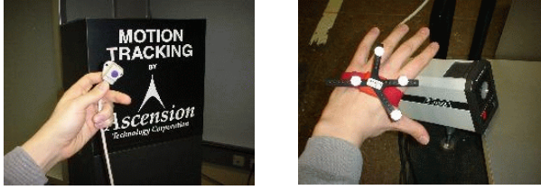
Fig. 1. Motion tracking devices: active sensor-based (left) and passive marker-based (right). (from [58])
